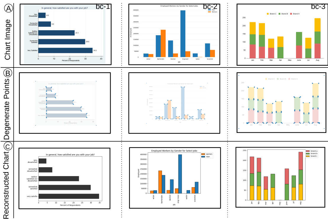
Figure FC5.4: Use of degenerate points in T_{V\text{-ad}} field for data extraction from images of multi-series bar charts, and validated using chart reconstruction. (A) Input images of charts. (B) Visualization of the pixels corresponding to degenerate points based on C_l and C_p values of T_{V\text{-ad}} at the corners of bar/bin for and near the center of scatterpoint, (C) The reconstructed charts from the extracted data for the input images.
